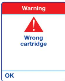
This warning message indicates that a wrong cartridge has been inserted.
