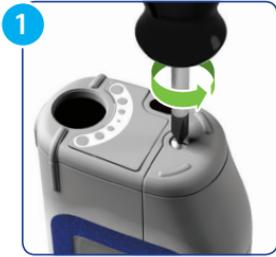
Unscrew the battery cover with a screwdriver.
