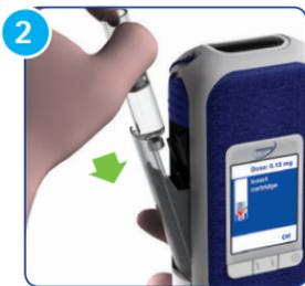
Place a new cartridge into the cartridge holder, making sure the metal tip is pointing down.
