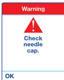
This warning indicates that the device has detected an issue with the needle cap attachment or detachment.
