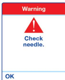
This warning indicates that an error occurred during the needle attachment or detachment sequence.
