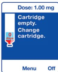
If, when you press the **Start** button, the cartridge is empty or has insufficient content for one injection, your easypod® will display **Cartridge empty. Change cartridge** and the cartridge content will be **0** and shown in red.
