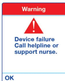
This warning indicates a permanent software or hardware error and the device needs to be returned.
