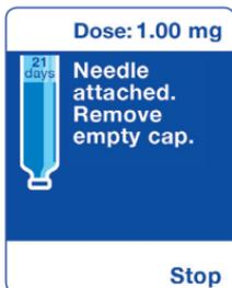
When device screen displays **Remove empty cap**, remove it by pushing it sideways until it detaches and can be withdrawn. Do not pull it straight down as this action may damage your easypod®.
