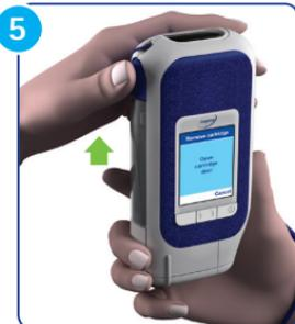
Slide the cartridge door button up to open it and remove the cartridge.
