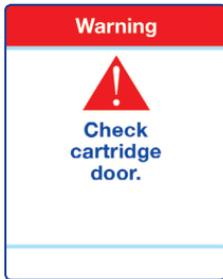
This warning indicates that the cartridge door is incorrectly closed.
