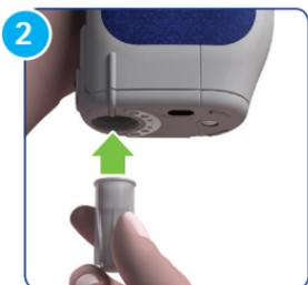
When device screen displays **Insert new needle**, push the needle cap, containing the needle, straight into the needle cavity until it clicks into place. Let go of the needle cap during the needle attachment.
