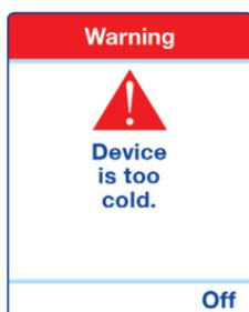
This warning indicates that the device temperature is below 4°C (39°F) to avoid potential malfunctioning.
