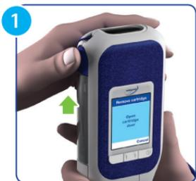
Open the cartridge door by sliding the cartridge door button upwards.
