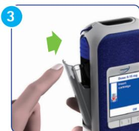
Push the cartridge door closed until it clicks shut. It will beep once when ready. You can start the injection by pressing **Start**.
