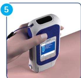
When the injection is complete the green injection button light turns off and your easypod® beeps twice.
